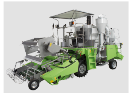
Delta with tine cloth pick-up device
