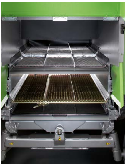
Shakers with double sieve system
