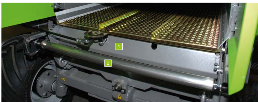
1 Electrical adjustable sieve setting 2 Grain loss sensor
