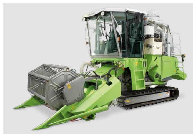
Delta with full track system for rice harvesting
