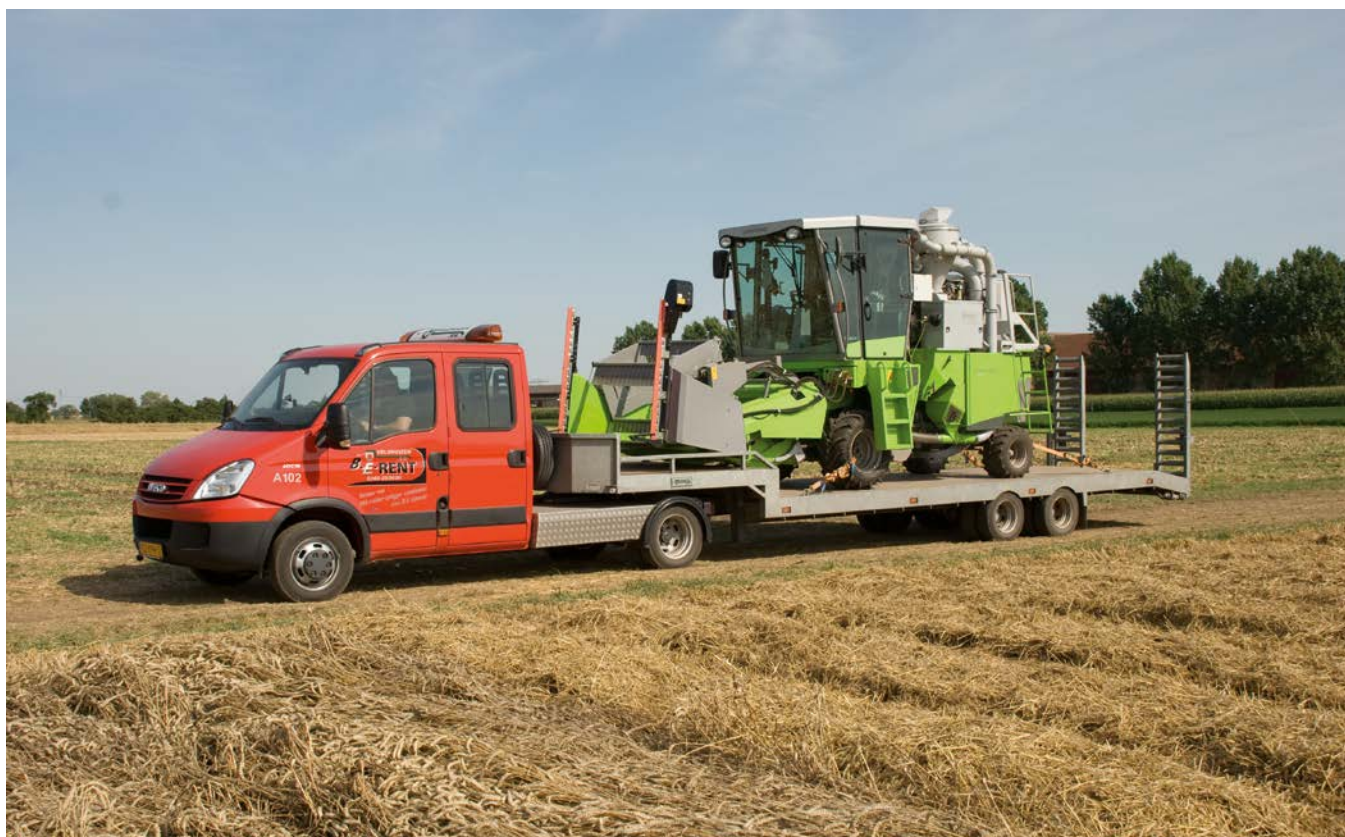
Thanks to the compact construction, the machine is easy to transport without removing components (maximum transport height: 2950 mm)
