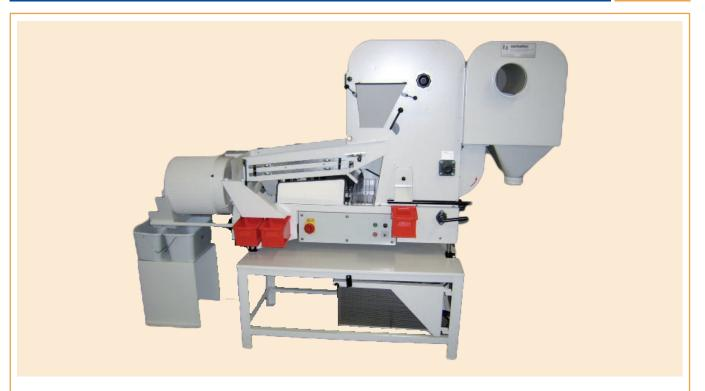
The **Petkus MP200** is a precision laboratory grade machine that meets all the requirements of a hemp seed cleaning machine, performing all functions, including stick and stem removal, based on a maximal capacity of 200 kg/h.
