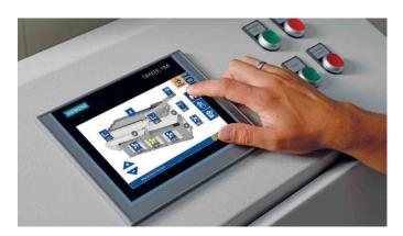
Recipe management, airflow, table angle, in-feed and vibration speed can all be adjusted with the user friendly touch panel. All settings can be saved allowing for exceptional and repeatable sorting results.
